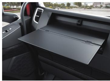
A folding table is integrated in the dashboard on the co-driver's side.
