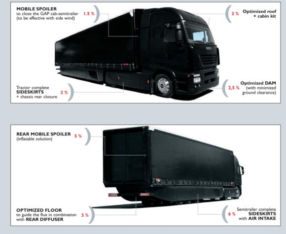
The results of the analysis, realised into Transport Concept, show significant improvements to the power loss due to aerodynamic drag, results that manifest themselves into energy and hence fuel consumption savings.
