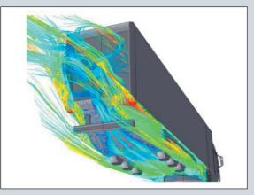
Application of tractor and semitrailer side skirts and a profiled under floor of the semitrailer contribute to a highly managed airflow beneath and around the vehicle.
