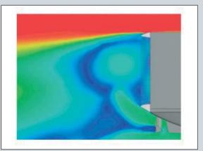
Similarly, an inflatable spoiler applied to the top and sides of the semitrailer rear door provides a managed slipstream to reduce aerodynamic drag.
