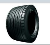
Compared to twin 315/70R22.5 tyres for the drive axle, Transport Concept uses super wide 495/45R22.5 drive axle tyres and reduces the rolling resistance by up to 4%
