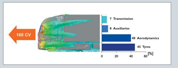
The power required to move a modern commercial vehicle along the road is quite modest. Ascending a gradient and acceleration pose greater power demands, however.
