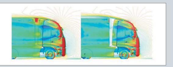
Studying the aerodynamic effects of the gap between the tractor and semitrailer. Transport Concept uses an innovative inflatable filler system to close the gap. Such a system is applicable to many semitrailer types and does not impede coupling and decoupling of the semitrailer.
