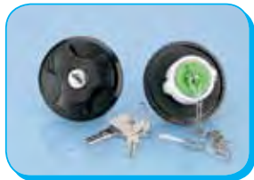
DAILY DAILY CITY VAN Cap with key ø72.5 for bayonet filler neck internal ø40. PN 2993927
