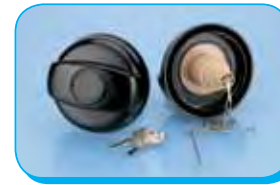
TRUCKS WITH PLASTIC FILLER NECK 80 P.6 DAILY CITY DAILY, TURBODAILY EUROCARGO TECTOR 60 → I80 E Screw cap with key ø103 for plastic filler neck M80 x 6. PN 500025735
