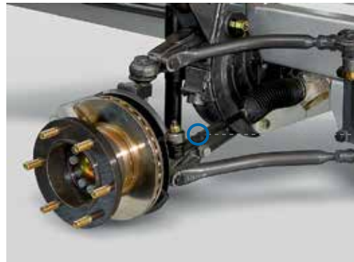
REINFORCED FRONT SUSPENSION WITH TORSION BAR
