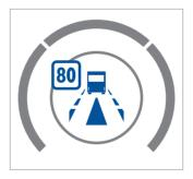
ACC Adaptive Cruise Control Keeps vehicle speed constant at the level selected by the driver. If a safe distance behind the vehicle in front is not maintained, the system activates the engine brake, retarder and (if necessary) the service brake.
