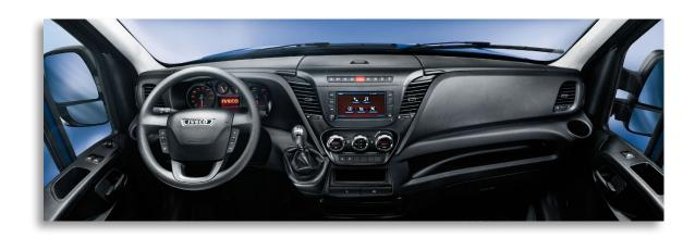
Specifically, all controls and storage pockets were designed with the idea of making them easy to reach from the driving position, including **five closed compartments**, **three cup holders**, as well as tailor-made compartments for everyday items, such as mobile phones and tablets.
