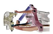
The new **QUAD LEAF front suspension** is based on a double quadrilateral arrangement with traverse leaf springs that produces excellent results in terms of containing dimensions and masses. This new front suspension, standard for all models up to 3.5 tonnes, is the best combination between the characteristics of the two previous versions thanks to several characteristics:
