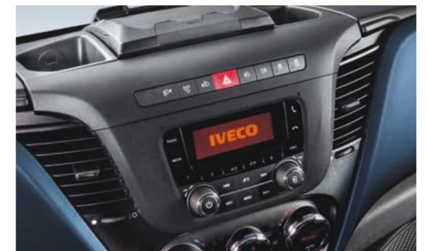
The new **DAB radio** integrated in the dashboard offers all the main DAB and FM features: for example, you can select the radio station by name, read the title of the programme or song you are listening to, set it to receive traffic and weather announcements, and pre-set up to 15 stations, to name a few.
