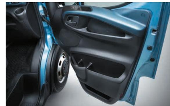
The door panel has been redesigned with an open compartment where, for example, you can store the first aid kit. The cab offers up to 18 practical storage compartments so that you can keep all your personal and working materials close at hand and organised.
