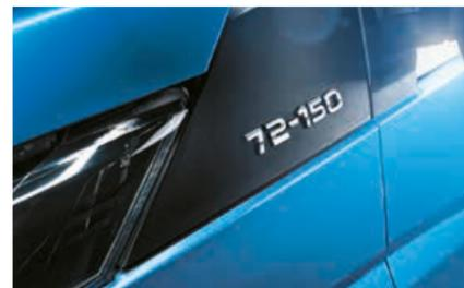
The Daily marking system is simple and intuitive: the code states the gross vehicle weight (in quintals) and the power (in hp).
