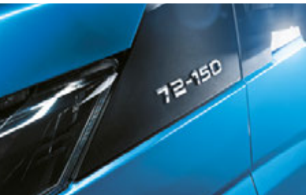
The Daily marking system is simple and intuitive: the code states the gross vehicle weight (in quintals) and the power (in hp).
