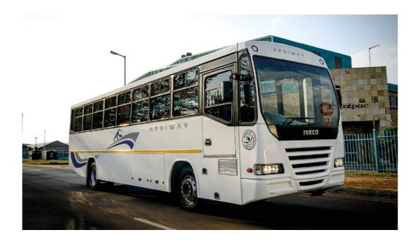
lveco 26.28M 6x2 front engine bus chassis with manual transmission fitted with the AFRIWAY bus bodywork.
