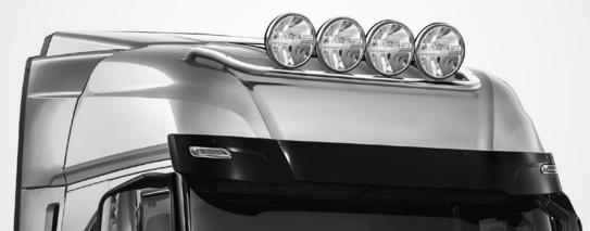
**SKY LIGHT High roof.** With LED cable for 6 lights, 6 fixed type holders, 5 white LEDs. Stainless steel, 60mm.
