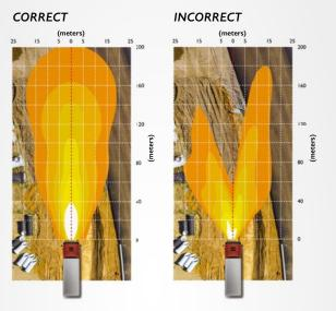
**Off-road illumination.** To ensure optimum visibility when working with headlamps on they need to be positioned correctly in order to provide an intense and precise source of luminous power – this is the only way to guarantee your comfort and safety while also taking the stress out of driving.
