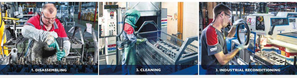
All cores are completely disassembled for inspection.
