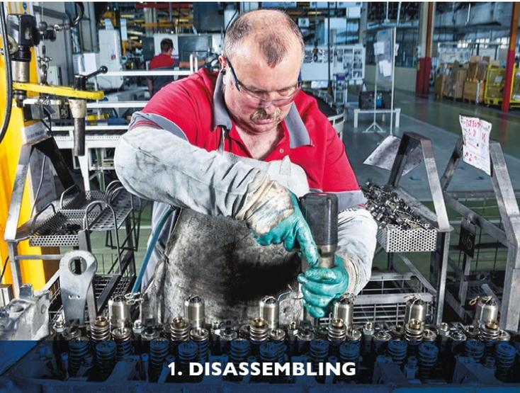
All cores are completely disassembled for inspection.
