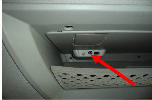
Figure 2 - Location of the USB connector on the upper shell
