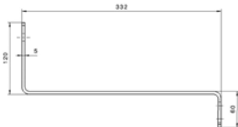
MATERIAL: ABNT/SAE/AISI/ASTM 1010
