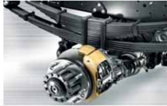
Disc brakes for the 9 to 12 t models. (10 t 4x4 versions with disc/drum braking system).
