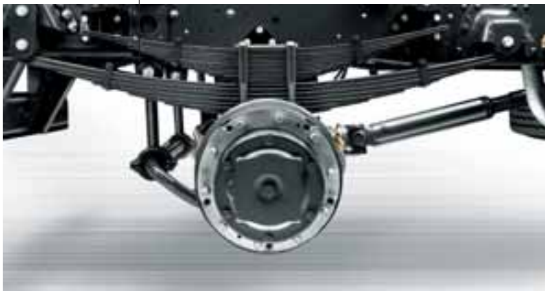
Semi-elliptical rear suspension. A solution designed for heavy use.
