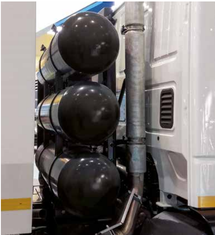
Rack behind the cab 420 litres / Up to 300km
