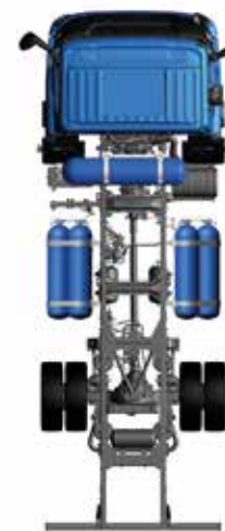
Standard layout + rack behind the cab 900 litres / Up to 750km
